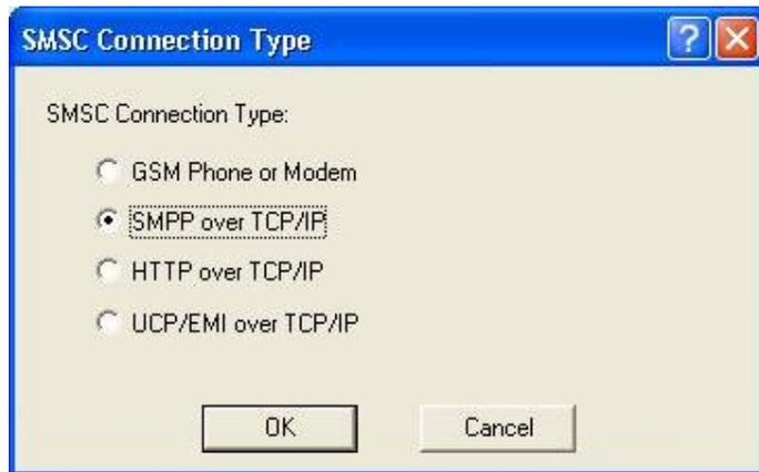
Figure 9 – Image from NowSMS showing the available connection types
