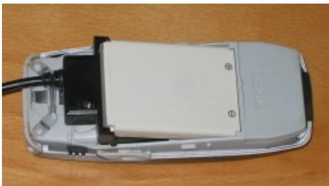
Figure 8 – Nokia 3310 with F-BUS cable attached
