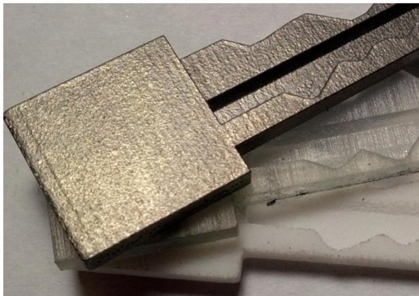
(From bottom to top, picture shows low resolution plastic, high resolution plastic, and titanium.)
