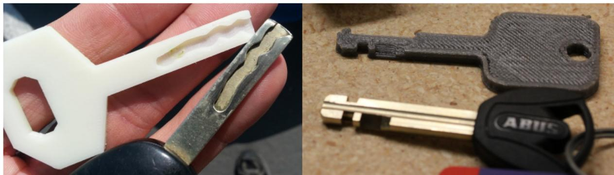
**Figure:** A 3D printed car key, by Ryan Weaving, and a 3D printed disc detainer key, by Nirav Patel.
